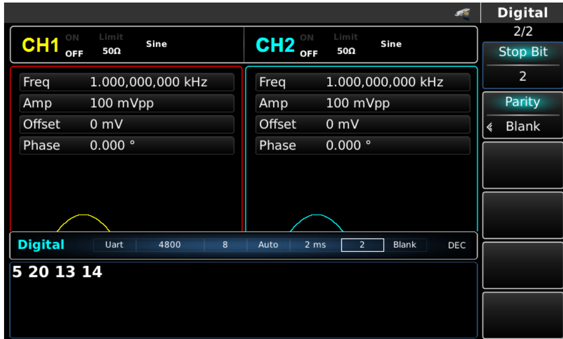
Figure 4- 162 Set stop bit
