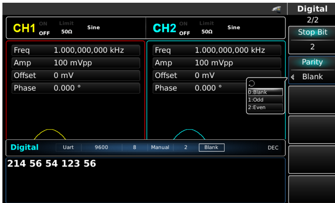
Figure 4- 156 Set check bit
