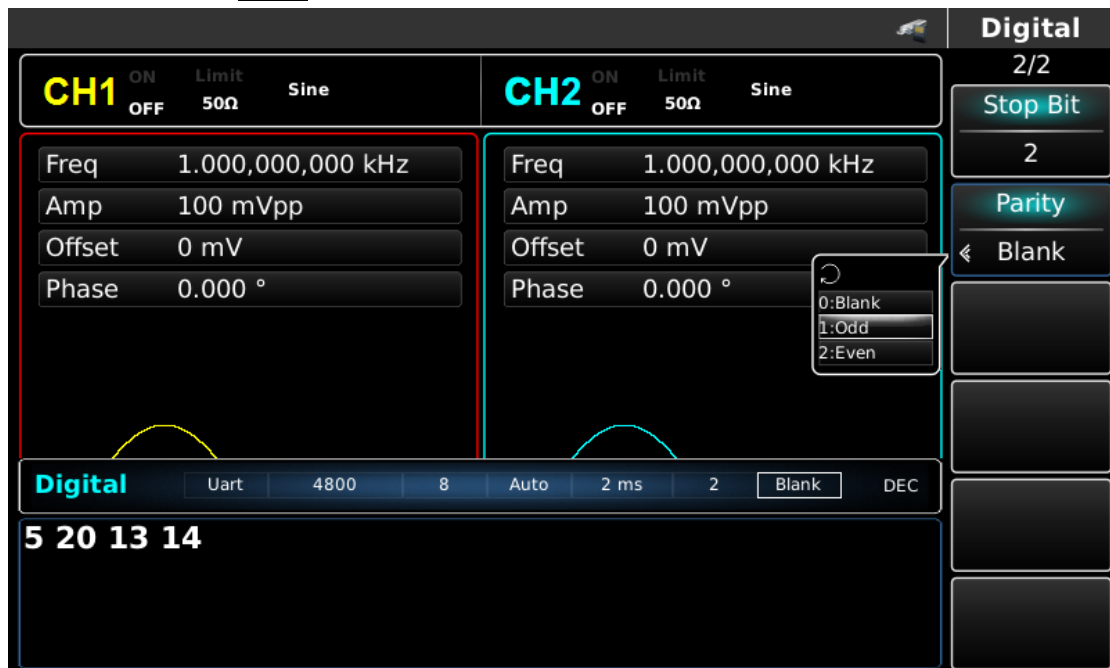
Figure 4- 163 Set check bit
