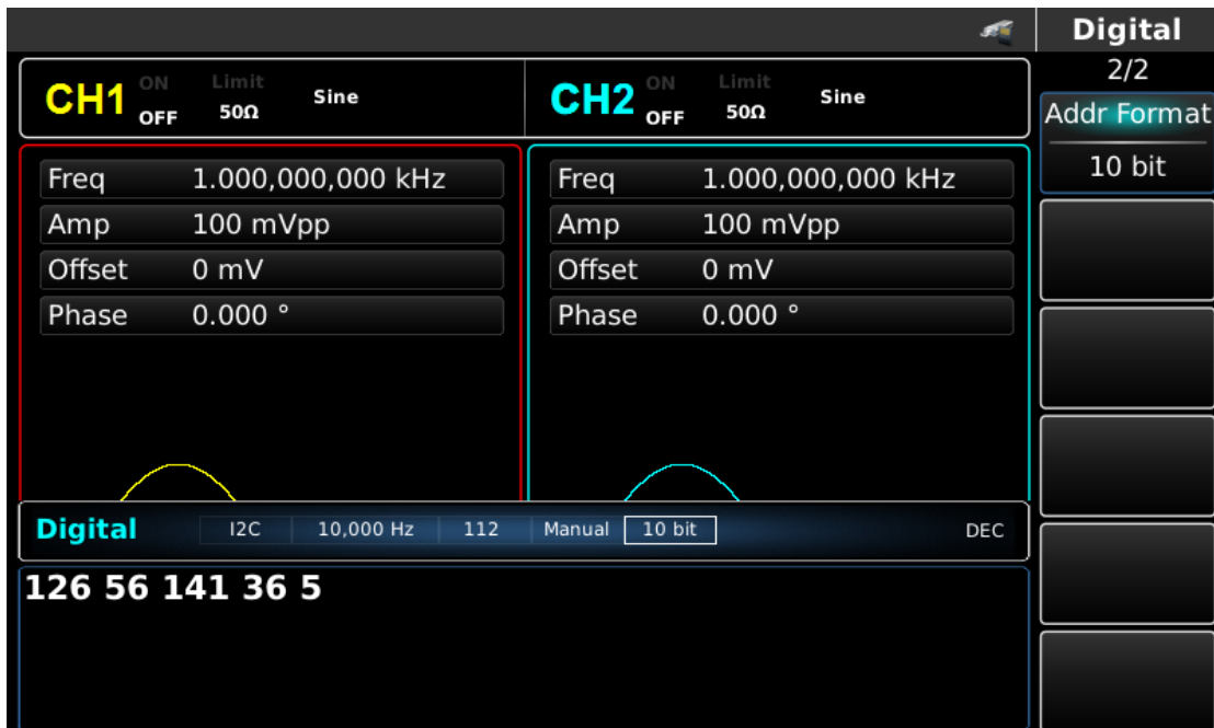
Figure 4- 173 Set 10-bit address
